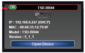
Once the correct DSP unit is determined select the correct box under the Map Physical Device menu in the Project View. When Mapped the DSP block in the Project View will become opaque.
