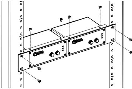
6. **TSD-RRMK Optional Rear Rack Mounting Kit** - For complete flexibility in mounting a TSD or TSD external power supplies the optional TSD-RRMK is available. The TSD-RRMK can support mounting of either two larger TSDs with external power supplies or up to 4 TSD models. **Note:** Only use the included M3 x 4mm screws as other screws may be too long and will cause internal damage to the TSD.
