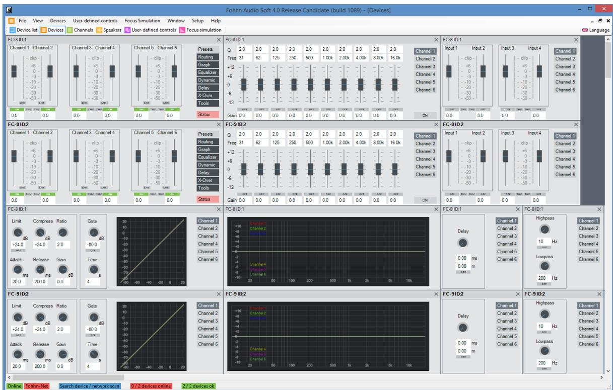
At the same time, **Fohhn Audio Soft** also enables the management and control of up to 254 active **Fohhn** devices, giving you constant feedback on both the status of the connected devices and their respective parameter values.
