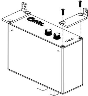
2. TSD-RMK 19" Width Rack Mount Kit - For 19" rack mounting, Atlas Sound offers an optional rack mount kit, the TSD-RMK. This rack mount kit can support up to four TSD units. The kit includes three blank panels designed to fill any unused slots. Use the included hardware to mount the TSD into the rack mount kit using the top mount screw holes on the TSD.
