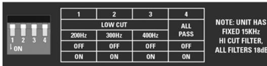
Dip Switch # 1 - 200Hz Low Cut, place switch in the down position to activate the filter.
