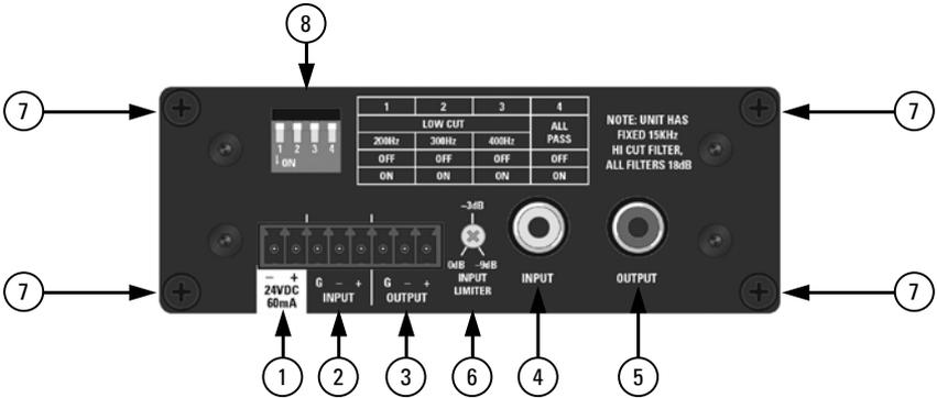
TSD Input/Output connections are removable for easy system wiring. The connectors have a 3.5mm pitch between pins.
