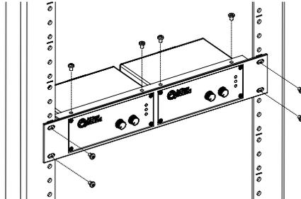
4. TSD-RRMK Rear Rack Mounting Kit - For complete flexibility in mounting a TSD or TSD external power supplies the optional TSD-RRMK is available. The TSD-RRMK can support mounting of either two larger TSDs with external power supplies or up to 4 TSD models. **Note:** Only use the included M3 x 4mm screws as other screws may be too long and will cause internal damage to the TSD.
