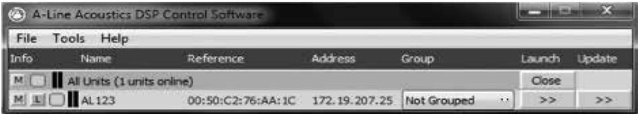
5. Click the [>>]; the update process will begin. Wait until the process is completed. Do not unplug or disconnect the AL123A-B unit from the network.
