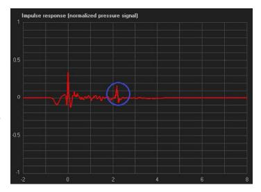
As a consequence of the windowing process, the computed IR is not accurate in the low frequency range: it is not possible to estimate the frequency response below the reciprocal of the analisys time interval, due to the time-frequency duality. So, to avoid misleading view, the frequency response plot shows a dotted line below 200Hz.
