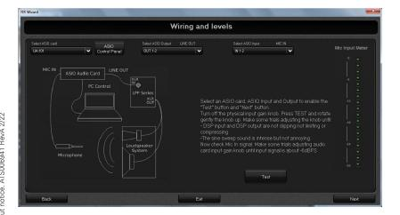
Connect an ASIO audio card to the PC where the FIR wizard is running, with its proper connection (USB, Firewire, etc.). Connect the (normally balanced) ASIO card output (XLR or TRS) to the balanced input (XLR) of the DSP device (e.g the LPP Controller).
