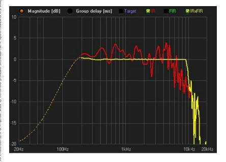
The graph below shows the group delay flattening effect (see the yellow curve), that is the main achievement of the FIR filter: a flat group delay means a linear phase of the sound system (the group delay is the derivative of the phase with respect to the frequency).
