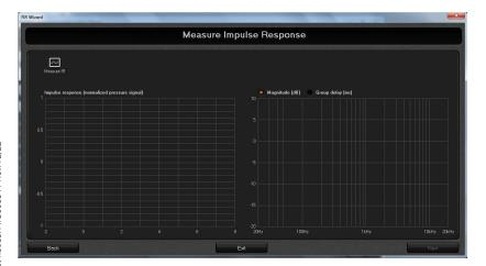
Clicking the "Measure IR" button at the top left of the screen, the measurement process starts and an activity progress bar shows the activity completion status. Wait in silence for the process completion. After the sine sweep, the Wizard starts the IR computation and the measured IR is plotted on the left graph with its peak centered on zero, while the magnitude and group delay frequency response is shown on the right graph.
