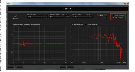
To start the verify process, click the "Measure" button at the top left of the screen and wait in silence. After the sine sweep completion, the new IR is computed and shown in the time/frequency domain plots. It is possible to compare the original and the compensated IR by acting on the "Before / After Correction" option button in the top right of the screen.
