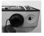
• Take external speaker wire connector from accessory package and unscrew the top cap.
