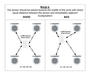
The reason behind this rule is to prevent similar issues encountered when considering Rule 1. If a sensor is located too close to any one speaker, the sound from that speaker could easily mask the ambient noise level from the sensor while an announcement is in progress. Since one sensor is usually placed in a zone with many loudspeakers, it is best to place the sensor where it is nearly equidistant from the immediately adjacent loudspeakers.
