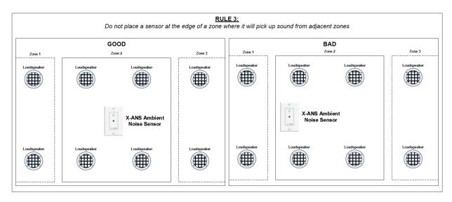
Placing the sensor too close to the edge of a zone can result in the level of the zone being adjusted based on program audio generated in the adjacent zone. Since the ANC algorithm only analyzes audio from the zone where the sensor resides, audio created by the PA system in an adjacent zone could cause the level of the parent zone to change. Placing the sensor in a centralized location within the zone will minimize the impact of audio from adjacent zones.
