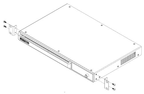
To rack mount the AZM4, remove included rack ear and ½ rack adapter and fasteners from hardware box and attach to each side.
