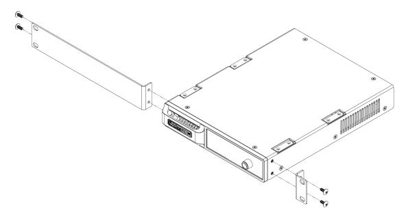
**Note:** The AZM4 is a ½-RU device and can be mounted in a side-by-side configuration using the AtlasIED part # PA702-RMK rack kit. It can also be combined with the IP power strip AtlasIED AP-S15HRIP.
