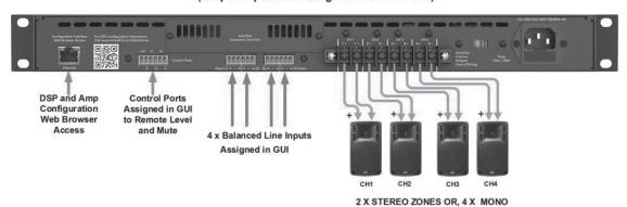
Configuration #3 <sup>2</sup> Channel 70V / 100V & <sup>2</sup> Channel  $4\Omega$  /  $8\Omega$
