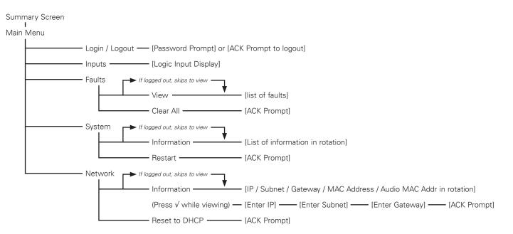
Figure: LCD Menu Structure
