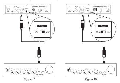
**Level Switch Setting:** When connecting to the LINE / AUX IN of a mixer / amplifier, switch to "LINE" position (Fig 18). DO NOT use the "MIC" position as they may not deliver a sufficient output level. When connecting to the "MIC IN" jack of a mixer / amplifier, switch to "MIC" position (Fig 19). Distortion may occur at the wrong level position.
