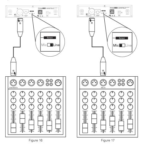
**Level Switch Setting:** When connecting to the LINE / AUX IN of a mixer / amplifier, switch to "LINE" position (Fig 16). DO NOT use the "MIC" position as they may not deliver a sufficient output level. When connecting to the "MIC IN" jack of a mixer / amplifier, switch to "MIC" position (Fig 17). Distortion may occur at the wrong level position.
