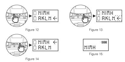
**Important:** Use only NiMH rechargeable batteries when using non-alkaline type batteries. Lithium Ion or other rechargeable batteries are not compatible with the MWBPT. NiMH must be selected when using rechargeable batteries. Never select AKLN (alkaline) when using rechargeable batteries. Incorrect battery selection will cause inaccurate battery information to be displayed.
