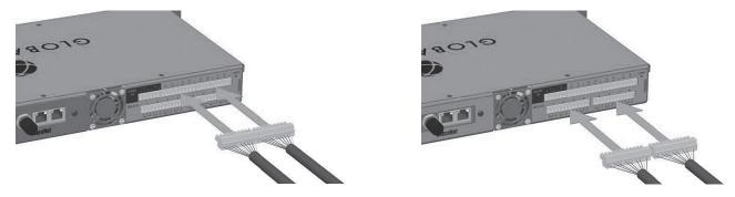
Each logic input is isolated and terminations are made by connecting the signal to the + terminal while using the – terminal for the return path to the signaling device. Pins 5 and 10 on each connector provide a reference to chassis ground. Refer to the image below for details on the logic and relay terminals.
