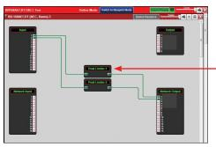
Note: Always add a limiter before the network output. Set the limiter threshold to OdBu to prevent clipping the input of the HPA amplifier.
