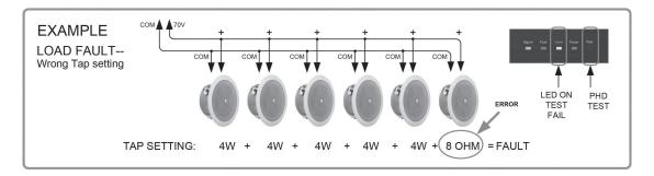
B. Check each speaker to be sure the load tap is set to the correct power setting. The total power tap selected of all the speakers combined should not exceed the amplifier's maximum power rating or a fault may occur.
