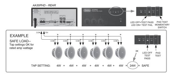
The Limit LED should never be constantly illuminated or damage may occur to the amplifier or sound system. If the Limit LED comes on steadily during use or during the PHD test there are a few common fault conditions to check if using a 70V distributed audio system.
