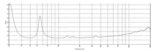
AHSUB15S-BSG Impedance (ohms) vs. Frequency
