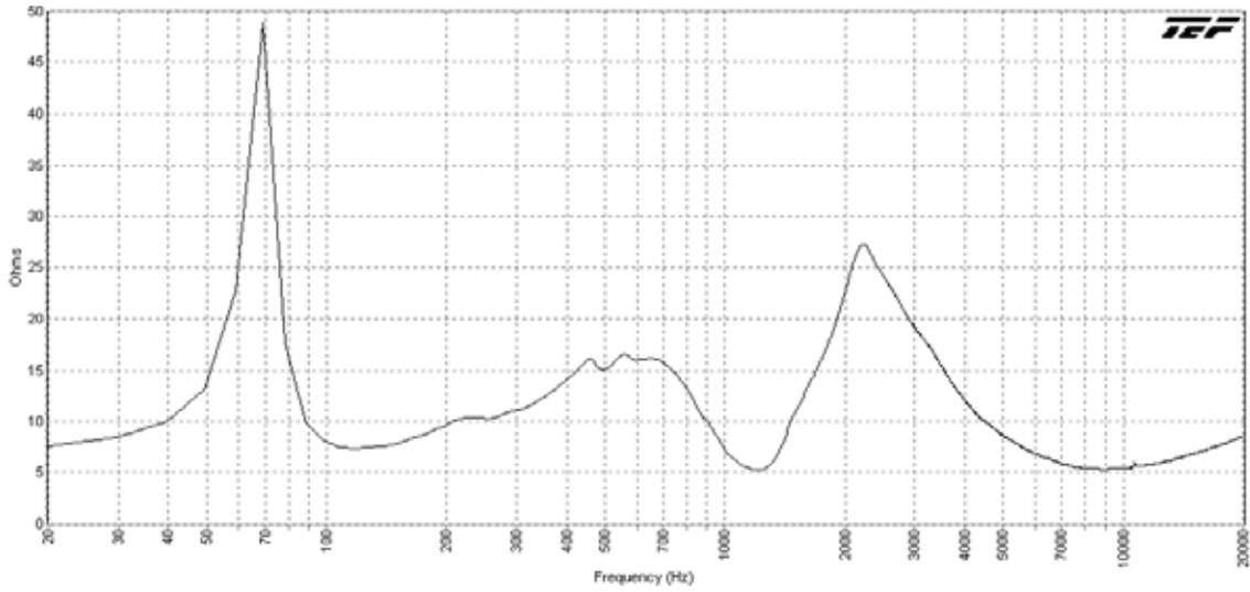
AH94-15-BSG Impedance (ohms) vs. Frequency
