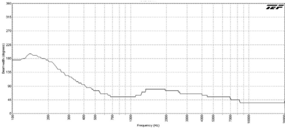
AH94-15-BSG Vertical Beamwidth (-6dB)
