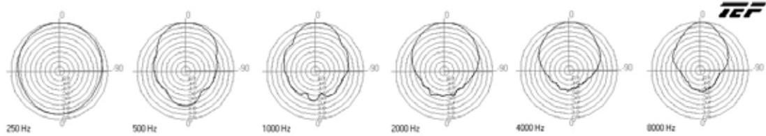
AH94-15-BSG Vertical Polars (Normalized to Zero on Axis) (-6dB)
