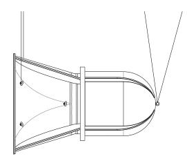
Note: Use of <sup>1</sup>/<sub>4</sub>" load rated wire rope is suggested to provide a static working load limit of 1400lbs (635kg) and moving load limit of 875lbs (397kg) per point. <sup>1</sup>/<sub>8</sub>" cable is not recommended as load limits are reduced to 400lbs (181kg) static, and 250lbs (113kg) moving.
