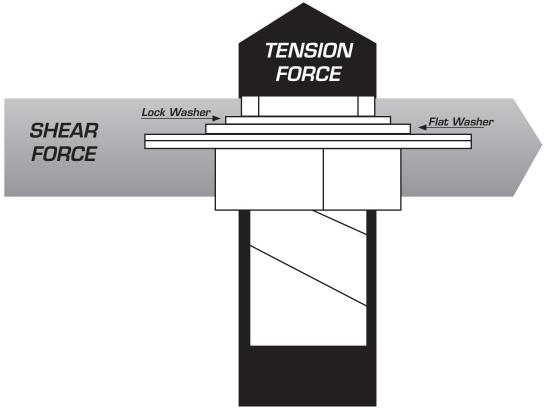
When mounting the AH speaker to a solid surface use the proper bolts, washers, and lock washers (Grade 5 minimum). Do not substitute mismatched bolts and washers.
