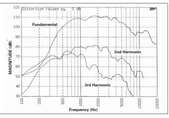
AP-15(T) (Harmonic Distortion - 1.5 watts @ 1 meter)
