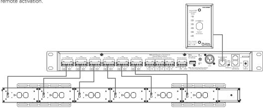
**Example 2:** 1 ECS-6RM<sup>8</sup> unit wired to 6 ECM-20 or ECM-20M modules in the ECM-RACEWY6 housing unit, using DCV 5-24V or a Switch for remote activation.
