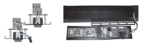
**Note:** The above figure shows the ECM wiring configuration of one 20A AC main line coming into an ECM-20M, then paralleling with an ECM-20 type module. It appears that the wiring is in series but the ECM Module In/Out terminals are in parallel on the PCB.
