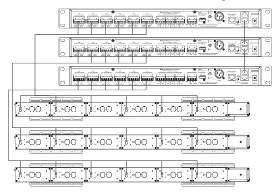
**Example 4:** 1 ECS-6RM<sup>B</sup> unit wired to 4 ECM-20 or ECM-20M modules in the ECM-RACEWY6 housing unit, and a separate ECM-15SH and ECM-20SH housing.
