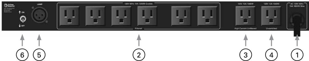
1. **AC Mains Input** – Connect the 9' (3m) power cord to a 15A 120VAC outlet to provide power to the AP-C15D.
