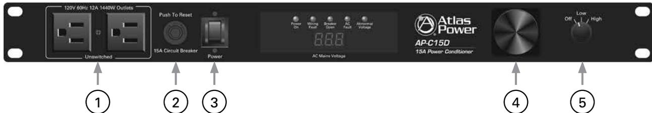
1. **Unswitched AC Outlet** – The two 120VAC outlets are always live when the AP-C15D power cord is plugged into an AC mains power source and voltage is present. **Note:** The AC mains power switch does not affect the Unswitched AC Outlets. The Unswitched Outlets are protected by the surge protection circuitry, but will not be shut off by the EVS circuit.
