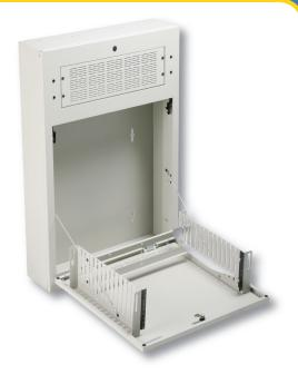
Doors can be opened to two positions—tilt-out for operation and by releasing side catches, the door will open to approximately 90° for equipment installation and maintenance. Units are furnished with two steel safety catch cables which suspend and hold doors at 90°.
