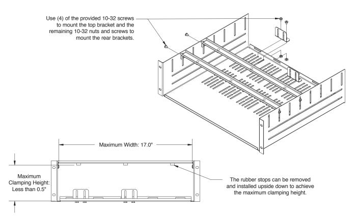
The rear brackets can be installed with the long flange up or down to provide greater flexibility.
