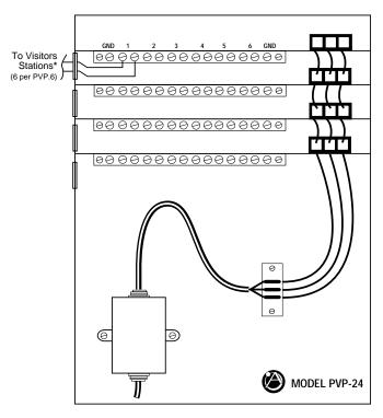
\*If sheilded cable is used, sheild can be connected to ground terminal at either end of terminal strip.
