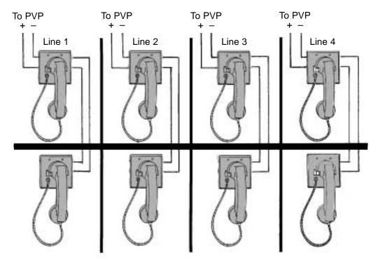
**Phone Stations:** Model CE-2-AC or Equivalent Connect Line to Terminals 3(+) and 5(-)
