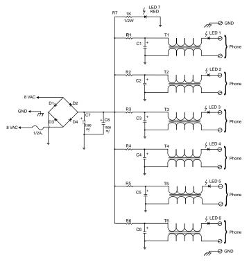
Resistors: R1-R-6  $47\Omega$ .½W Capacitors: C1-C6 470mf 35 V
