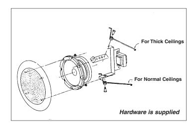
Note: For proper support, torsion spring grilles should not be used with 8" loudspeaker assemblies exceeding 5 lbs.
