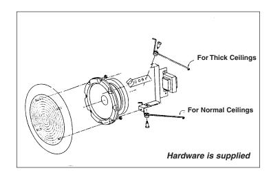
Note: For proper support, torsion spring grilles should not be used with 8" loudspeaker assemblies exceeding 5 lbs.
