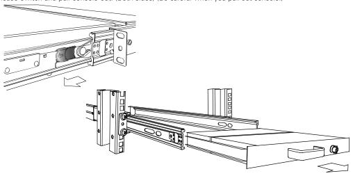
7. Push rail-lock switch on the rail and push rail back. (Both sides)
